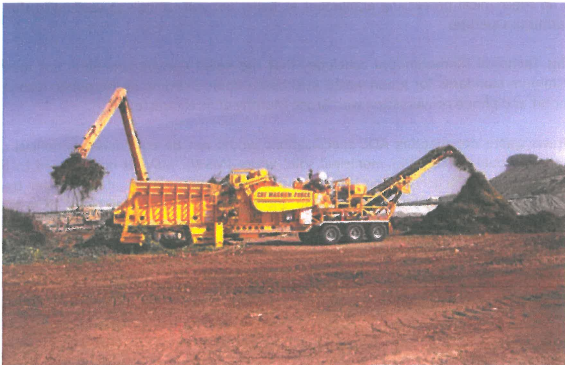
From Exhibit C – Figure 3. Unprocessed green waste (on left) is ground and stockpiled (on right)
