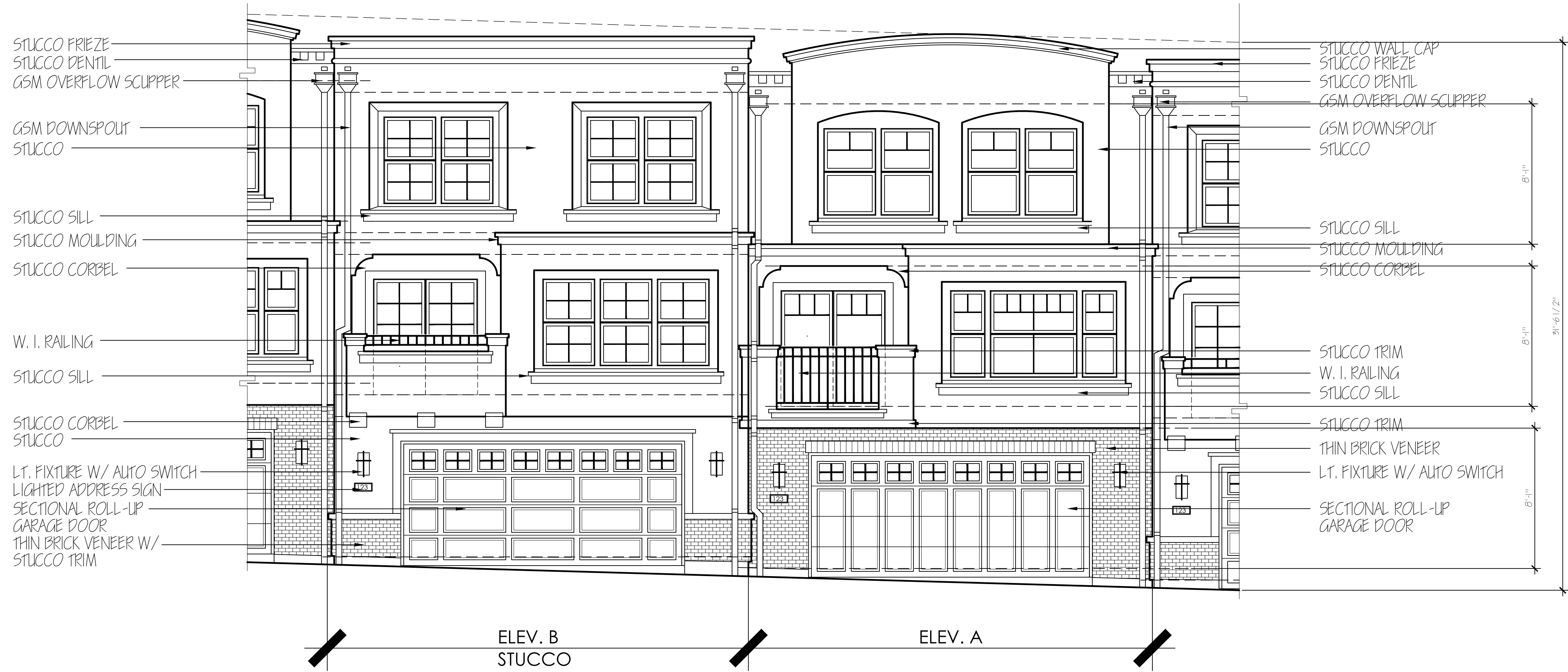
TYP. UNIT EXTERIOR ELEVATIONS
