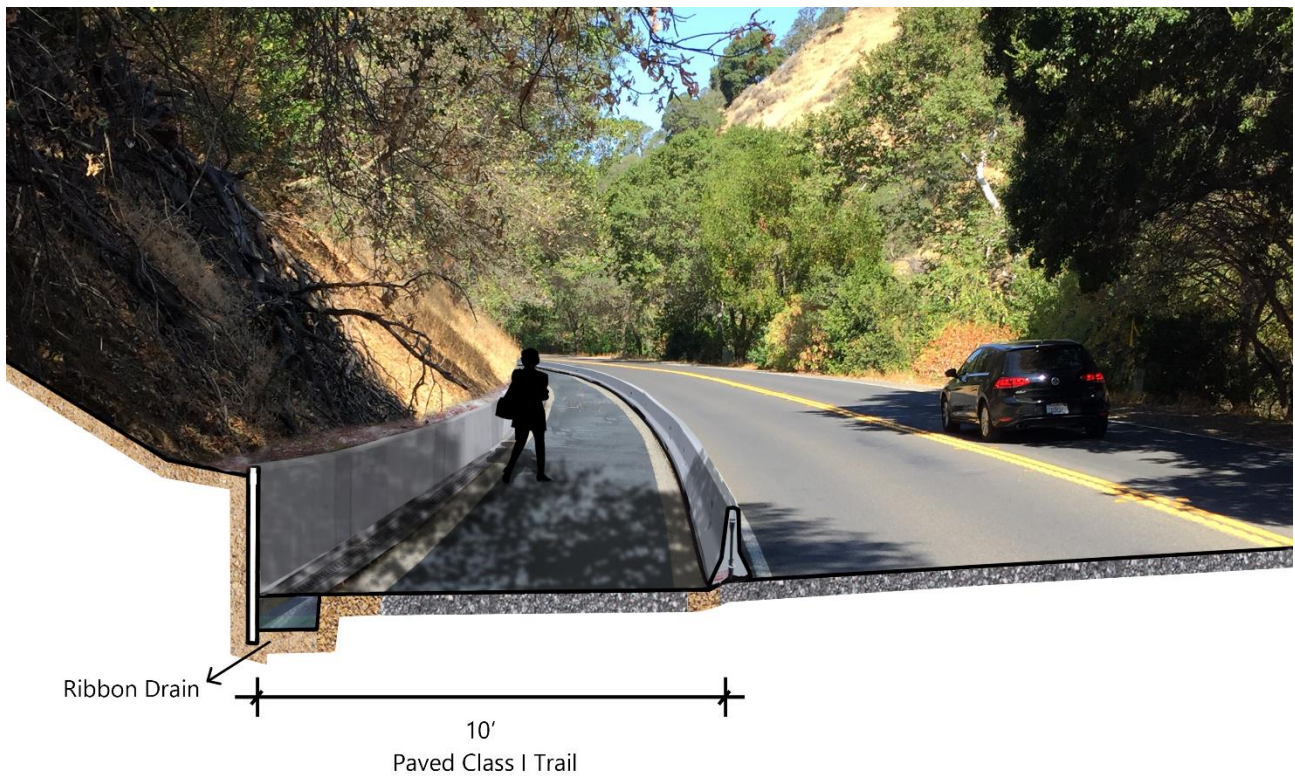
Figure 5-4. Trail in the ROW along base of steep hill
