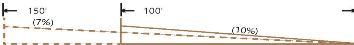
Figure 4-5. Change in length of trail needed to rise 10 feet at gradients of 7%, 10%
