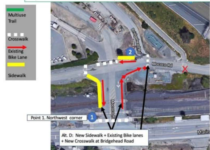
4.1 Pt. 1 Mococo Road /Marina Vista to Pt. 2 Bridgehead Rd. Alternative D: Modified Existing Alignment – Bike lanes and sidewalks Separate routes for bikes and pedestrians.
