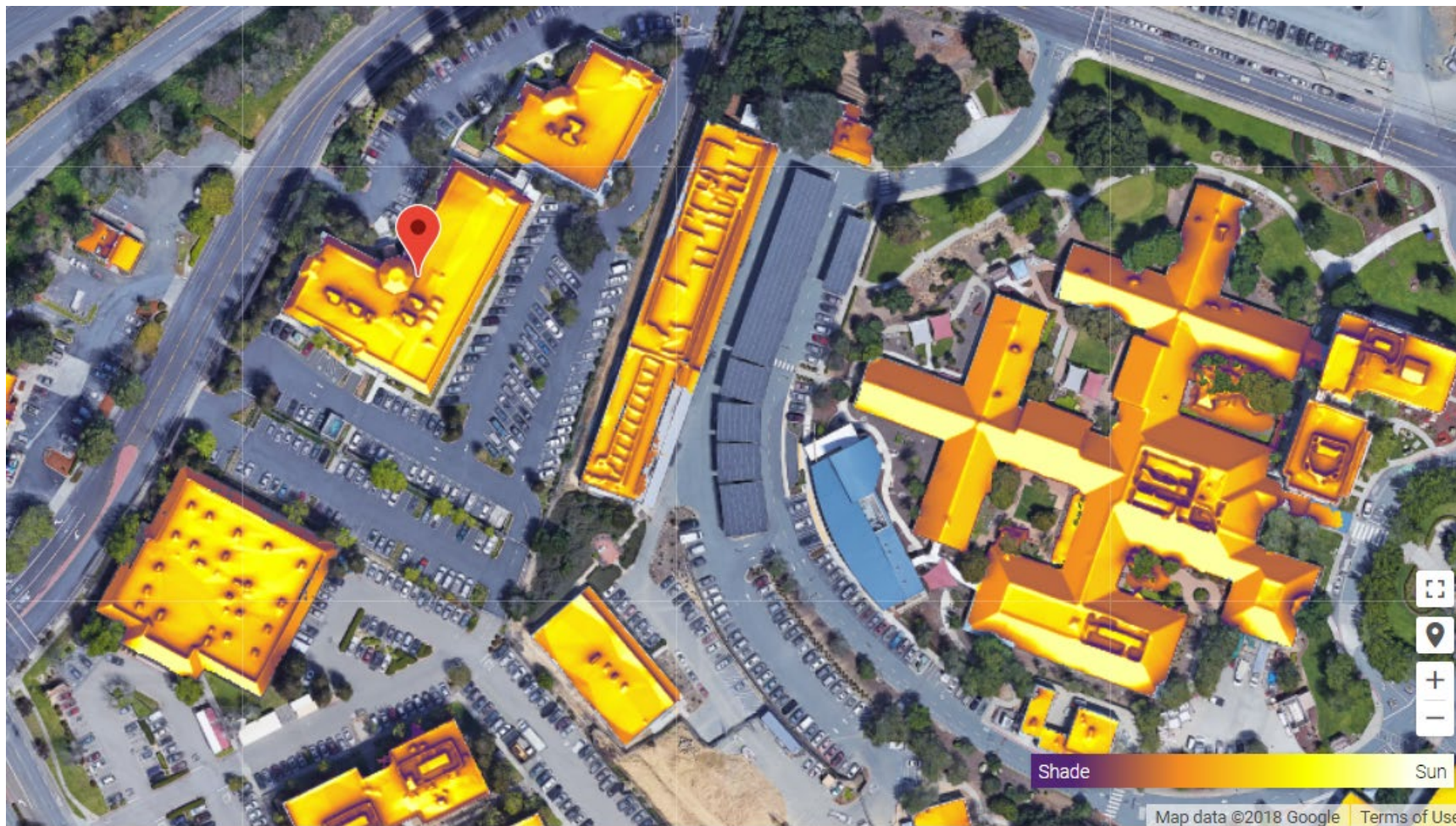
Figure 9. Zoomed in screenshot of Google Sunroof’s characterization of rooftop solar availability and shading at DCD’s offices and surrounding buildings in Martinez
