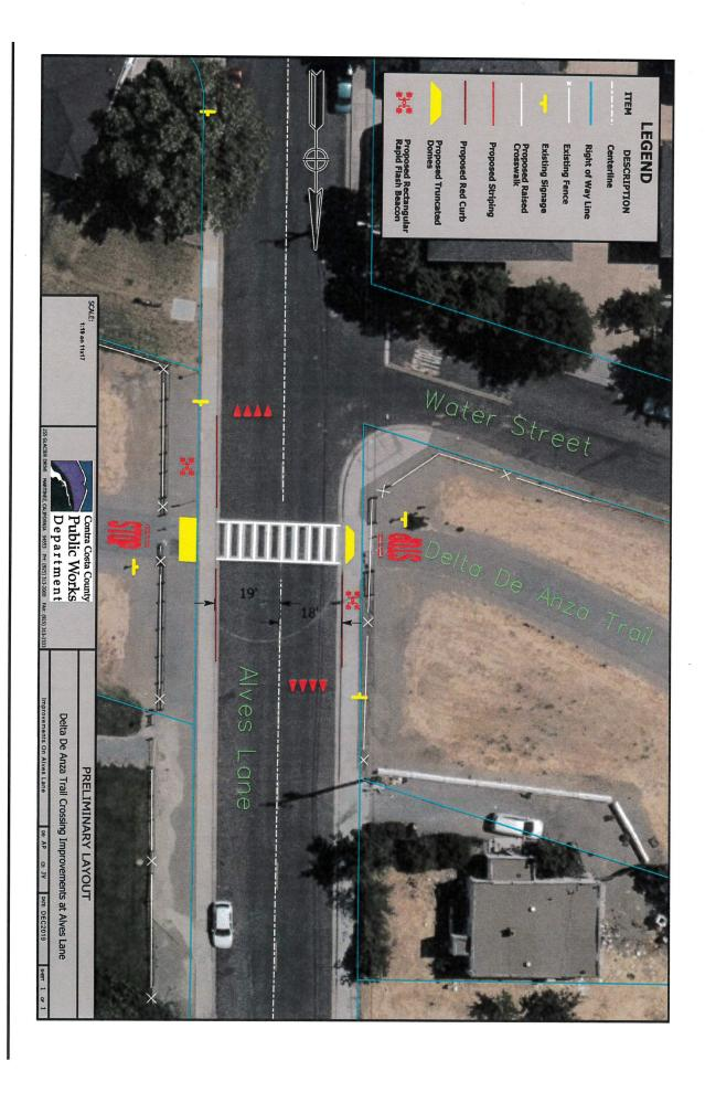
FIGURE 3: Proposed Layout Delta de Anza Trail Crossing Improvements at Alves Lane
