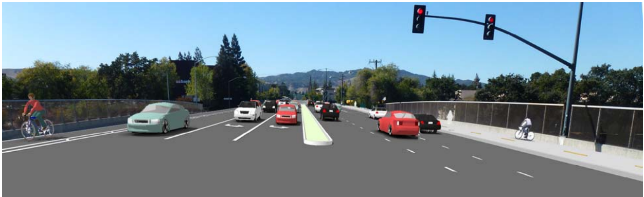
Figure 5-3: Concept 2 shared use path (north side) and buffered bike lane (south side) at I-680
