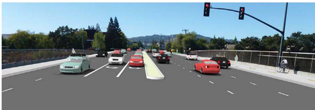
Figure 5-5: Concept 3 shared use path (north side) and sidewalk (south side) at I-680
