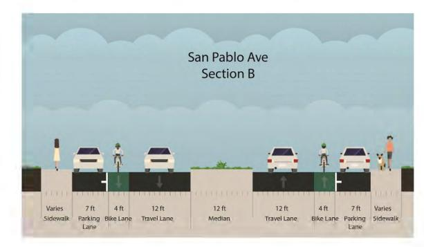
NOTE: BIKE LANE AND PARKING LANE ARE NARROWER THAN STANDARD. THIS MATCHES EXISTING CONDITIONS.
