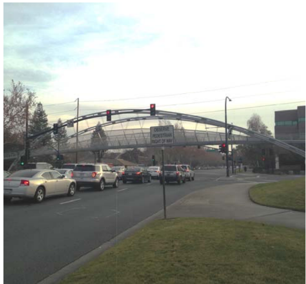
Photo 20 Treat Boulevard looking east toward Jones Road. A non-compliant MUTCD sign tells drivers to "observe pedestrian right of way."
