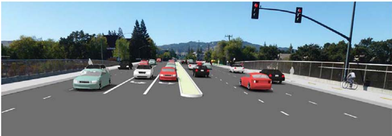
Figure 5-6: Concept 4 shared use path (north side) and sidewalk (south side) at I-680 (as per Concept 3)
