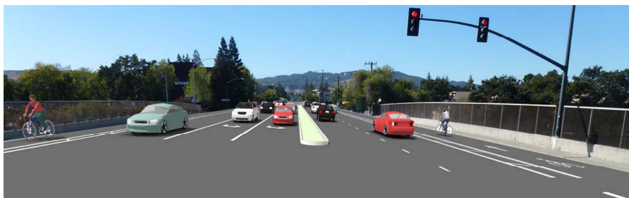
Figure 5-2: Concept 1B buffered bike lanes at I-680
