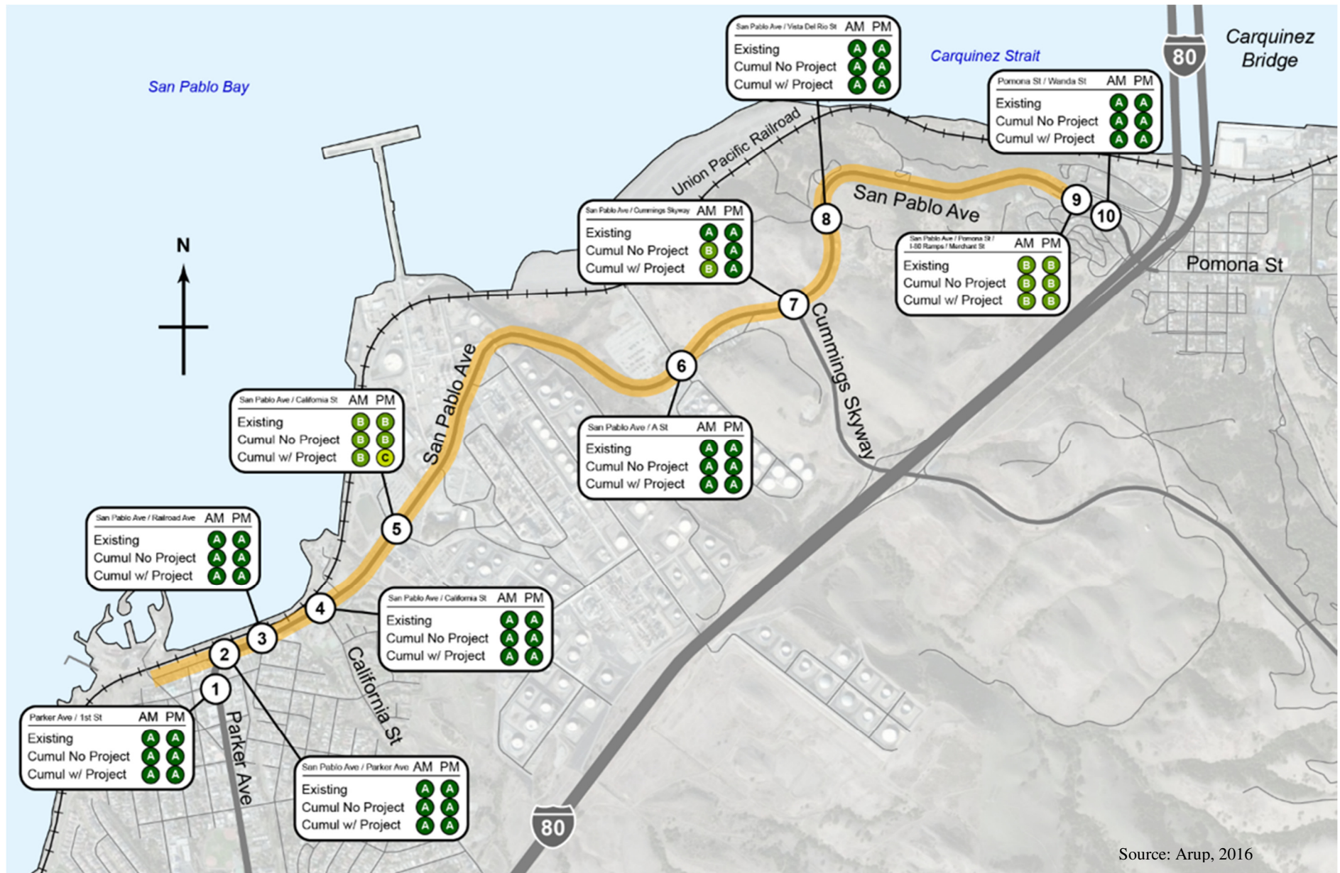
Figure 13: Intersection Traffic LOS Results
