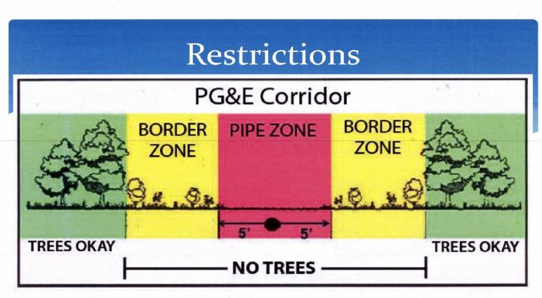
**Pipe Zone** the Pipe Zone is defined as the area that extends 5 feet from the edge of the pipe on both sides. Planting within this zone restricts vegetation to non-woody, low profile ground covers not to exceed 18 inches in height.
